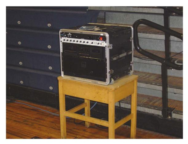
The Gator Rack is the portable component of the Expo Sound system. It is configured to be set up in various locations around the arena and to provide control of multiple microphones and audio inputs. The rack includes an 8-channel mixer, a CD/cassette player, one microphone and cable and an adapter for a computer or mp3 player. Up to 3 more microphones may be available upon request. Please inquire in advance.
